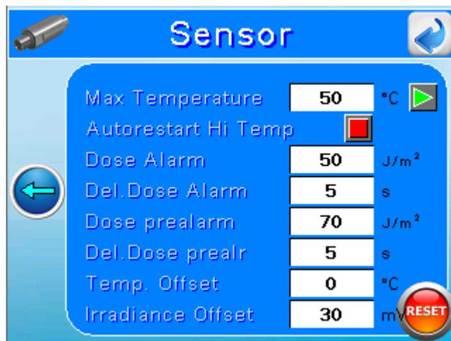
this screen allows to set alarm thresholds.
