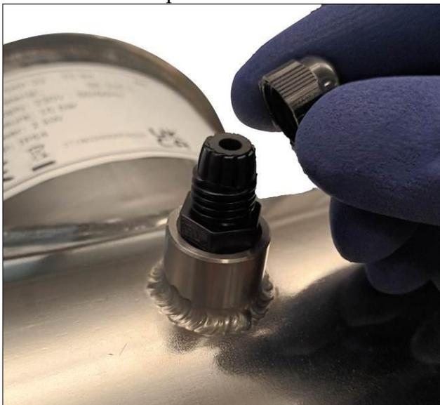
a) Remove the cable gland cap
