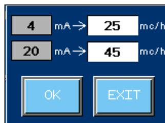
Associate the values 4 and 20 mA to the minimum and maximum flow rate input. Touching "OK", the user calibrates the 4/20 mA input.
