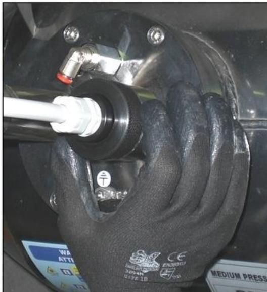
6 Screw the ring nuts on the sleeve bolts.
