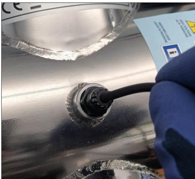
c) Make sure that the sensor element (at the end of the cable) is in contact with the bottom of the bush
