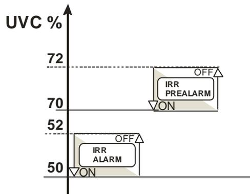
When Dose is below the alarm threshold, water can't be fully disinfected. To avoid this warning, clean the quartz containing lamps, replace lamps or improve water quality with an adequate pre-treatment.
