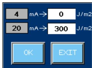
Associate the values 4 and 20 mA to the minimum and maximum Dose (Irradiance). Touching "OK", the user calibrates the 4/20 mA output.
