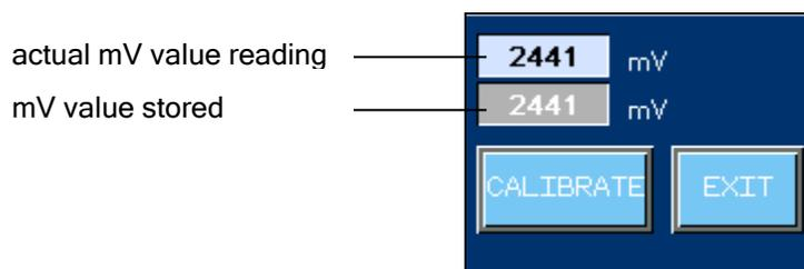
Touching on "CALIBRATE" the user confirms that the signal read by the sensor corresponds to 100% of the radiation of the lamps.
