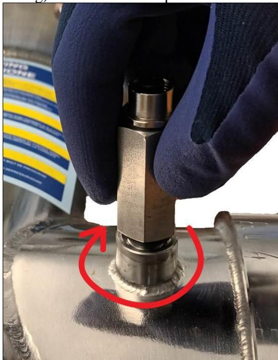
4. Install drain and vent valves.
