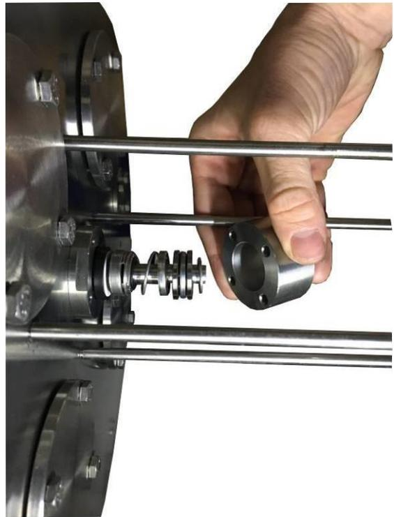
Using the screwdriver, remove the motor shaft seal and replace with the new one. Reassemble all and restart the UV system.
