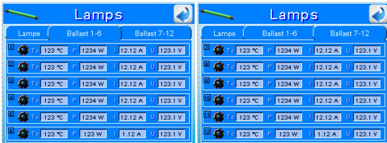
This screen shows the actual values of temperature, power, current and voltage of each lamp.
