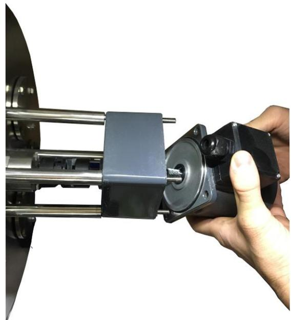
Unscrew the joint locking nut and extract it (Use Torx size 8).
