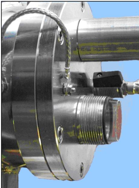
Insert the o-ring on the sleeve (point 8)
