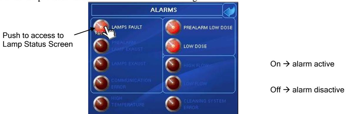
**LAMP FAULT** → Each lamp of the UV system is identified by a number. This message visualizes the lamp number which is not working.
