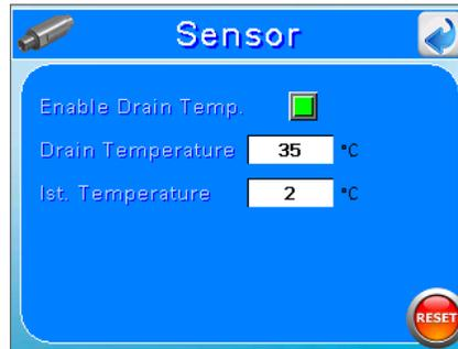
1. **Drain Temperature:** temperature value which causes activation of drain valve.
