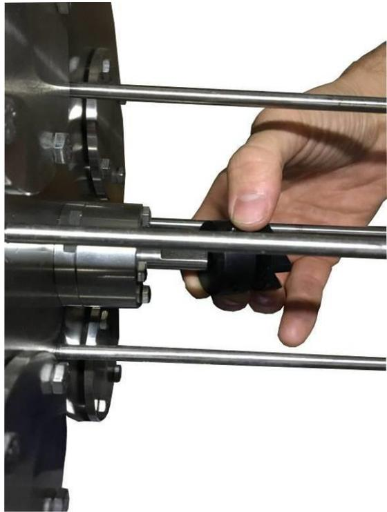
Remove seal housing by unscrewing its bolts (Use socket wrench size 8).
