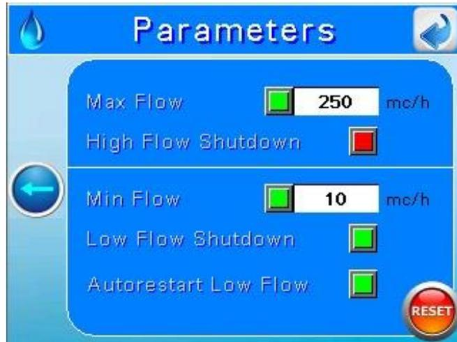
this screen allows to set alarm thresholds.
